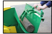
Log fix device on log saw
