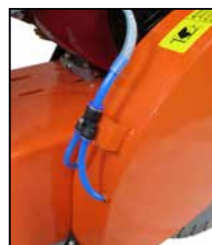
Double water pipe for cooling both side of blade
